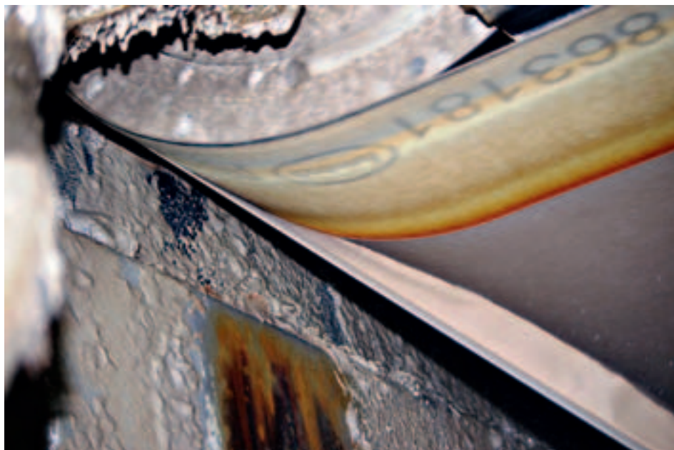
Fig. 3: This is the result of a properly functioning trim jet
