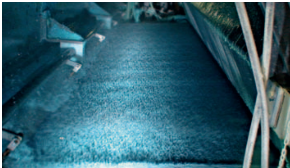
Fig. 1: A spot-pattern strobe light such as the Unilux Beacon provides enough light in the center area of the wire to monitor high-pressure jet sprays. Clear nozzles are required to produce a spray that will clean the wire after a production run and prevent contamination, which can result in defective product, on future runs
