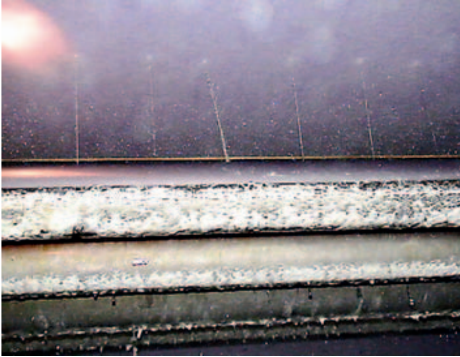
Fig. 5: Using the Unilux Beacon allows operators to see that the high-pressure shower is not working correctly. The shower is non-laminar or not aligned
