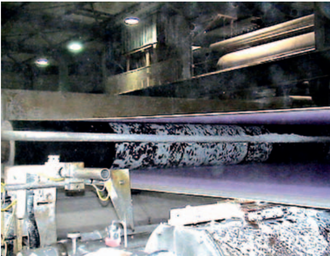
Fig. 6: The spot-pattern light from the Unilux Beacon shows the extent of plugging in the return rolls
