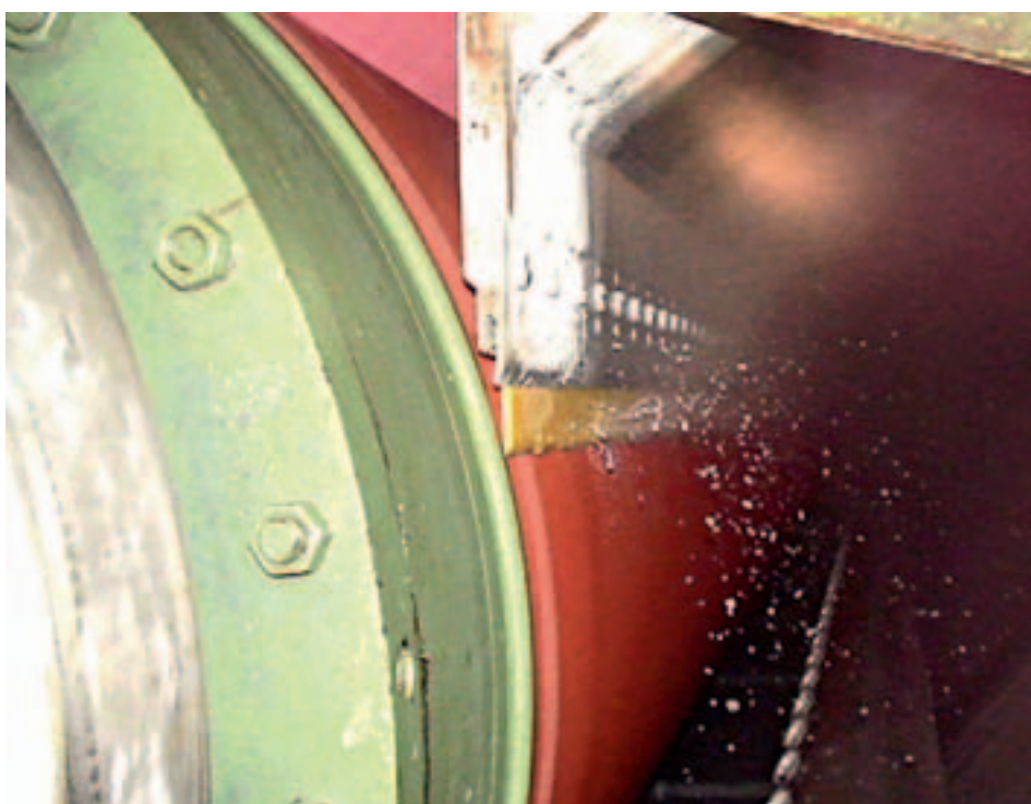
Fig. 4: The spot-pattern light from the Unixlux Beacon shows the dewatering at a press roll
