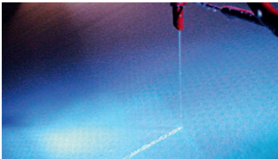
Fig. 2: The Unilux Beacon spot-pattern strobe light can show the efficiency of the web trimming process. Good lighting enables operators to observe trimming in more detail; keeping trimming within specifications can prevent many costly breaks
