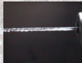
Turbulent jet at nozzle exit
