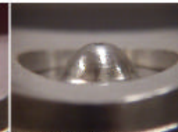
Nozzle above level of inner pipe wall
