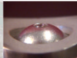
Nozzle above level of inner pipe wall
